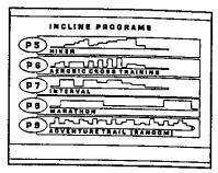
RANDOM program, P-9, will be different each time it is used.) The HIKER, AEROBIC CROSS TRAINING, and INTERVAL programs are 20 minutes long with 3-minute cool-down periods; the MARATHON program is 28 minutes long with a 1-minute cool-down period; the RANDOM program will last for 60 minutes, but can be stopped at any time. Follow the steps below to use an INCLINE program.
